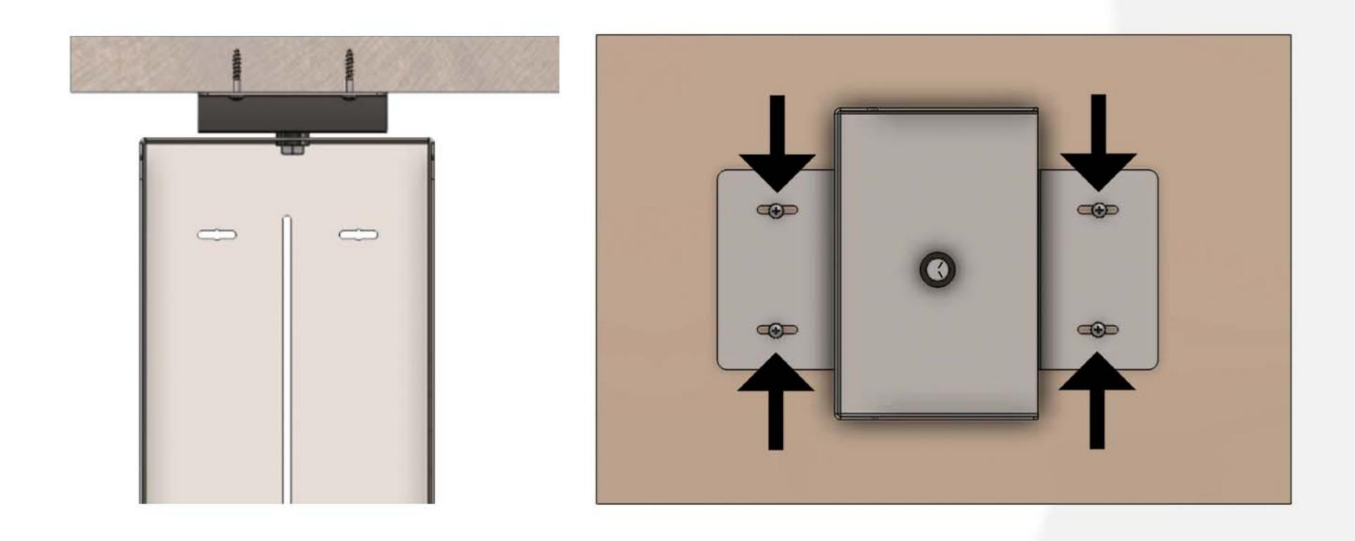
**Step 3**: Align Part-4 with Part-1 by determining the height of the computer and fasten the screws as shown in the below image.
