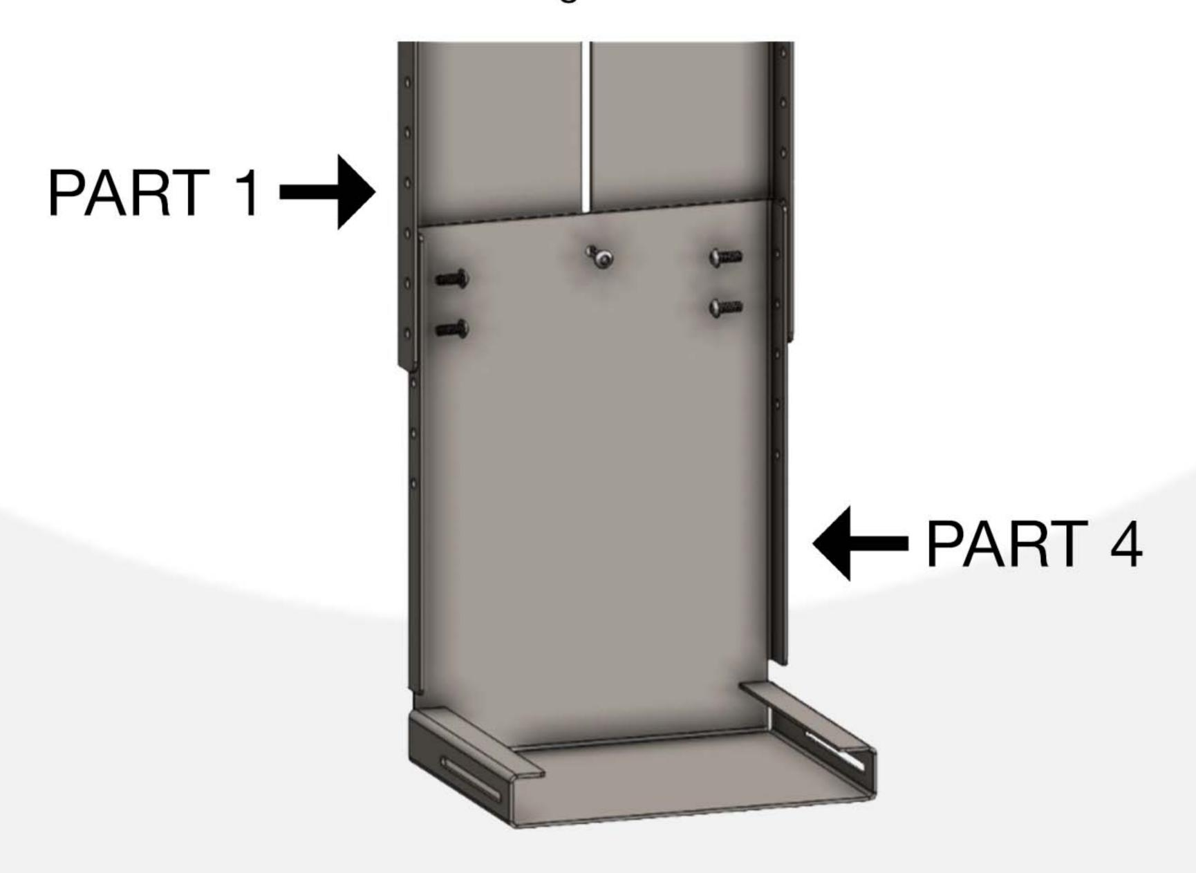
**Step 4**: Tighten the screws to keep the mount in place with the wing nuts provided.
